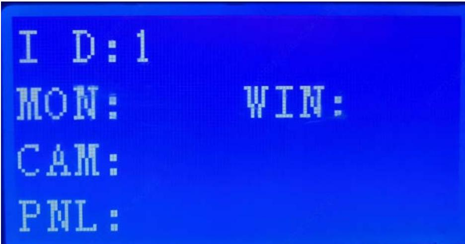
**Step 5 MON** and **WIN** do not have any meaning when the keyboard is used for NVR controlling.
