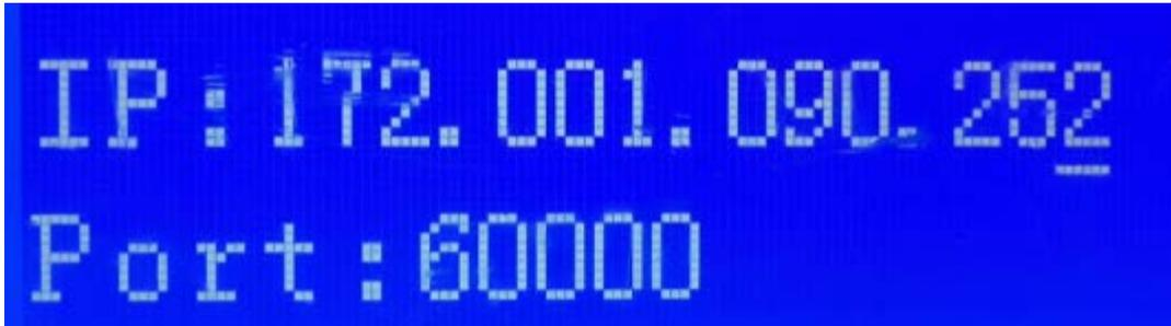
Press **Enter** and then **ESC** to save the configuration. The NVR has been added to the keyboard successfully.
