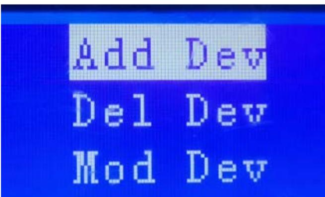
Set ID, name, device type and connection type like below, then press **Enter** and put in the IP address of NVR.
